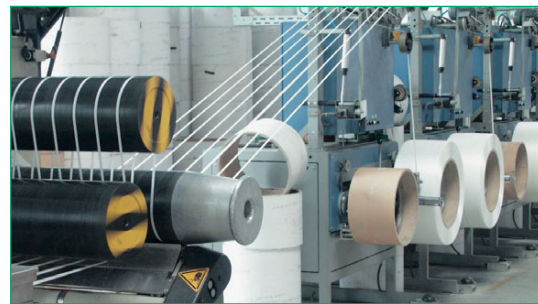
Fig. 4 Stretching process of ribs
